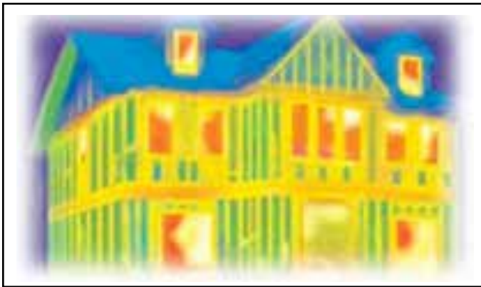
House with OSB and R-13 batts
