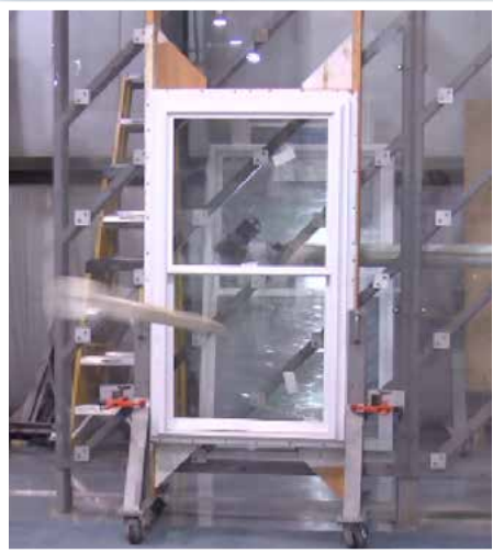
Missile Level D Impact Testing. In the initial part of the impact test, the window is shot with a 9-lb, 8-foot-long 2x4 projected out of a canon.
